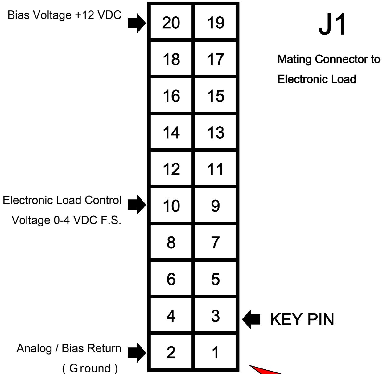
**NOTE:** If you have a connector with pin numbers stamped on the side, disregard the pin numbers stamped on the side of the connector.
