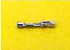
Step one, crimp the pin with no wires.
