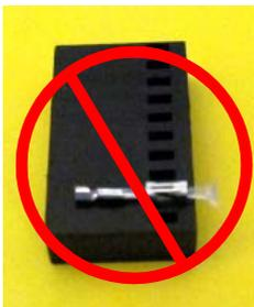
Do NOT stick the plastic key pin in the metal pin until the metal pin is in the connector....! The Plastic Pin is a one time insertion and CAN NOT be removed once it is inserted.
