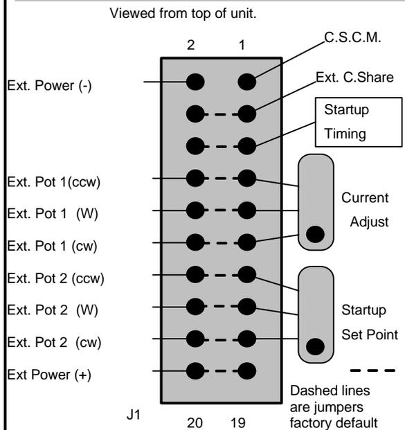
**Figure 3. Connector : Electrical Connections**
